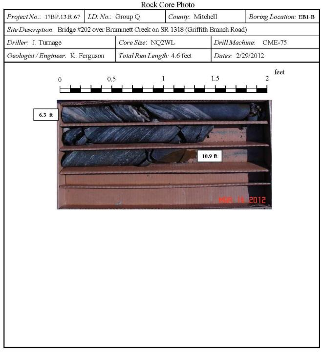
Notes: 1) Used NQ2 core barrel with wire line
